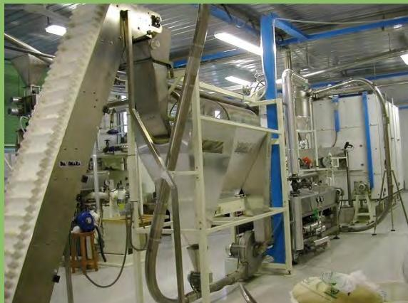
**Fig. 7** - Pilot plant for production of couscous (courtesy of Fava SpA, Ferrara, Italy).
