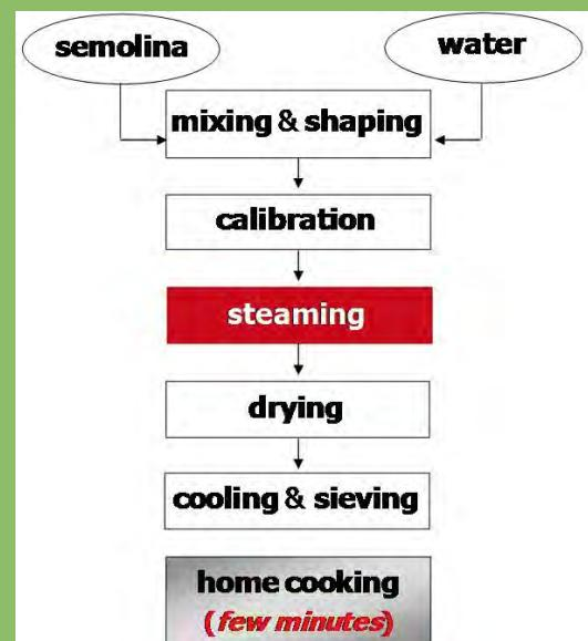
**Fig. 6** - Flow-sheet of industrial production of couscous.
