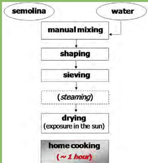
**Fig. 4** - Flow-sheet of artisan production of couscous.
